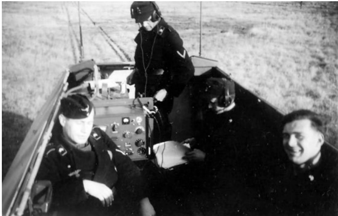
Figure 4: A period photograph of a Sd.Kfz. 251/3. Note the placement of the 80 W.S. on the front side of the radio rack. The absence of a frame antenna indicates that the remaining radio configuration was probably different. [© www.worldwarphotos.info]
