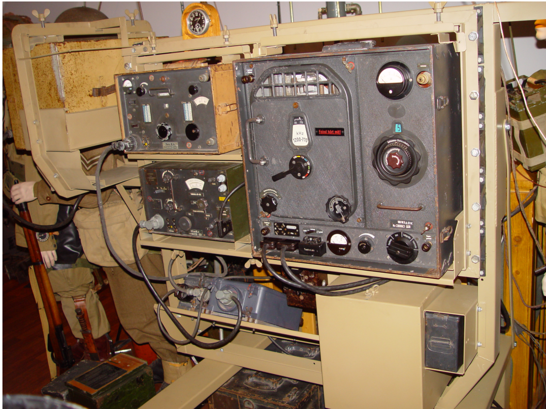
Figure 18: Right 3/4 view of the radio installation. The front view shows the Torn.E.b and 100 W.S. of the Fu11SE100 and the Mw.E.c of the Fu12SE80, the 80 W.S. is soon from the side on the far left of the picture.
