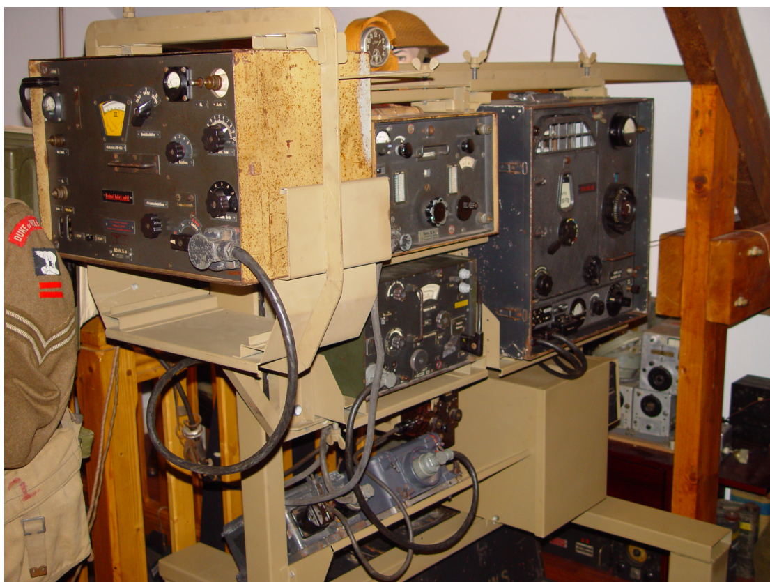
Figure 17: Left 3/4 view of the radio installation, showing the position of the 80 W.S. transmitter of the Fu12SE80.
