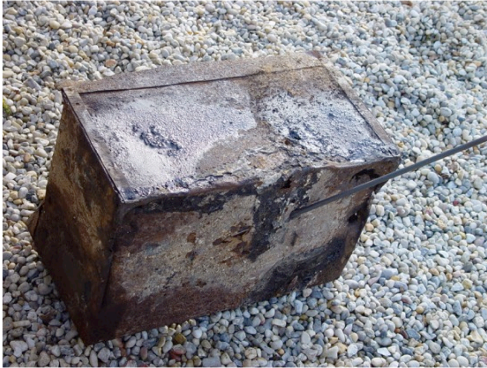
Figure 8: 80 W.S. case showing the approximate impact angle.
