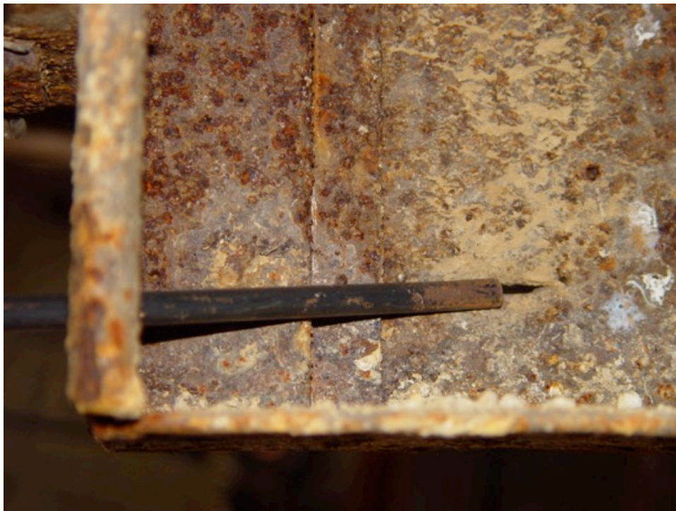
Figure 9: Approximate trajectory of bullet hitting the bottom tray of the 100 W.S. rack.
