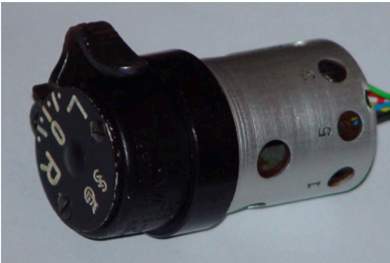
Figure 11: The "Richtungsgeber" was normally build into the control column with only the top black bit showing. It would be operated by pushing the slider to he left or right with the thumb
