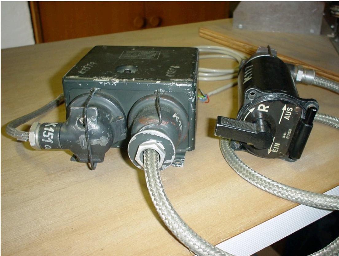
Figure 19: a Lrg 5 and LKW 5, Note the various "K" numbers painted on the components.
