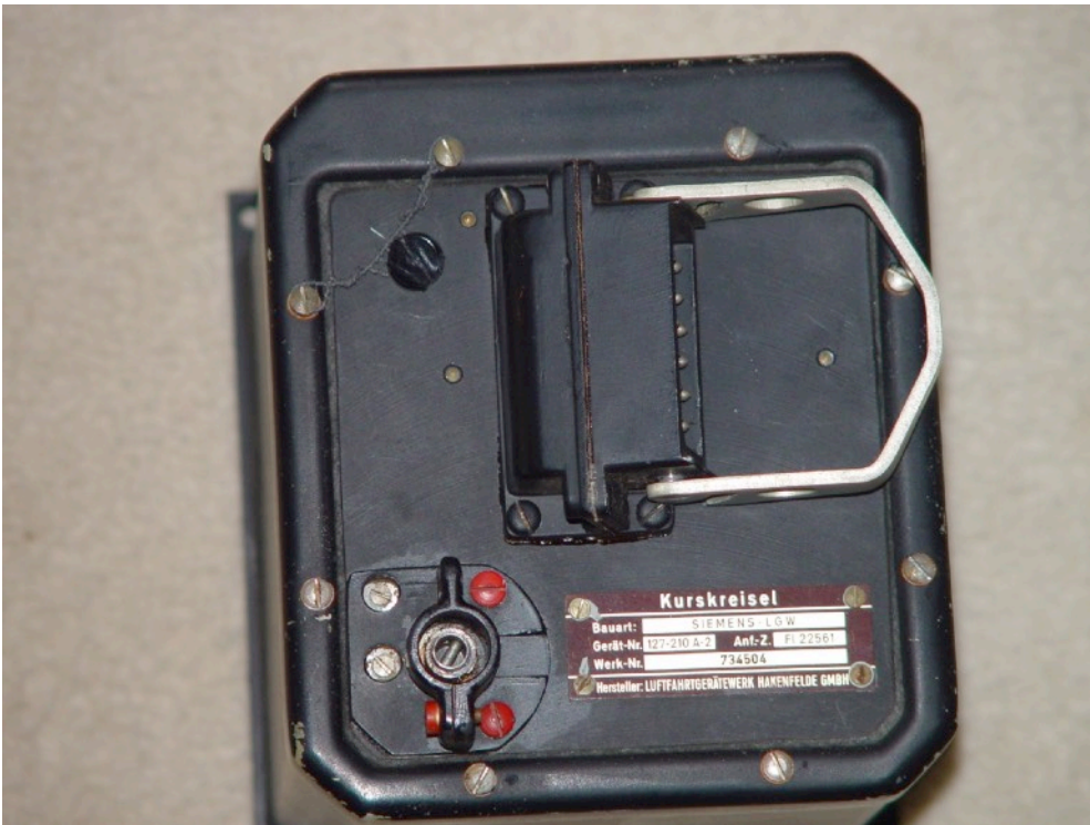
Figure 9: Rear view of the "Kurskreisel" showing the plug connection and bottom left the input shaft connected to the "Kursmotor"
