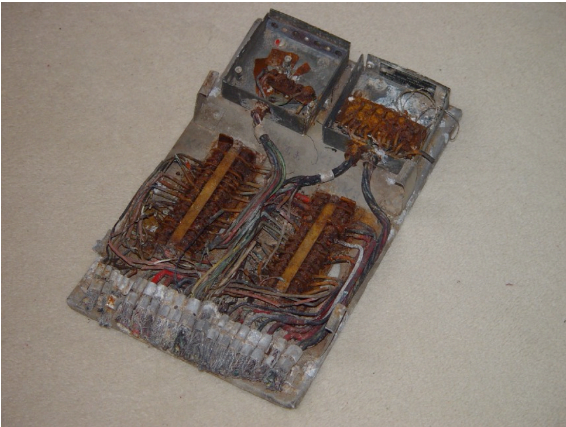
Figure 18: An original relic distribution board for the K4u autopilot. Note the remains of the "Widerstandkasten" on the far end
