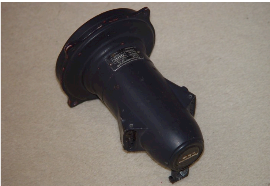
Figure 6: Back of the "Führerterchterkompass" showing the plug sockets and bottom rear the entry of the driveshaft of from the "Kursmotor"
