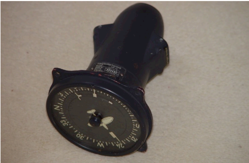
Figure 5: A Patin PKT/f3 "Führerterchterkompass". Note that this version has two plug sockets on each side of the instrument.
