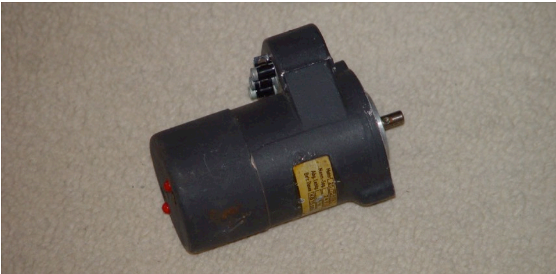
Figure 23: Dual winding series motor used to drive the turntable. These are normally used as an electric trim motor on the Fw 190.
