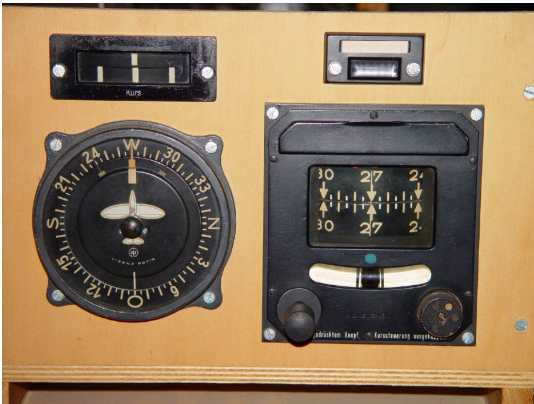
Figure 20: All the instruments are aligned on a course setting due West. The rudder should stay central.
