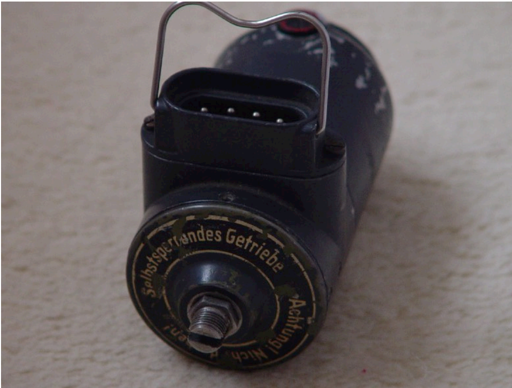
Figure 13: a "Kursmotor" . Note the warning that the output shaft should not be turned manually as the motor contains a self locking gear mechanism
