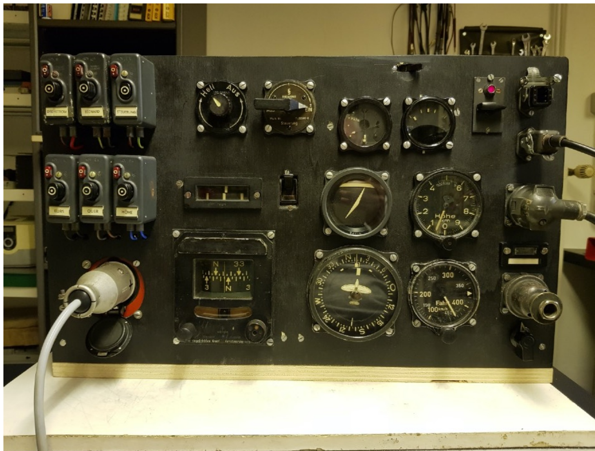
Fig. 19: The dashboard is now extended by a FuG 28 instrument (top right) and next to it an AFN2, for the blind landing described in the last chapter.
