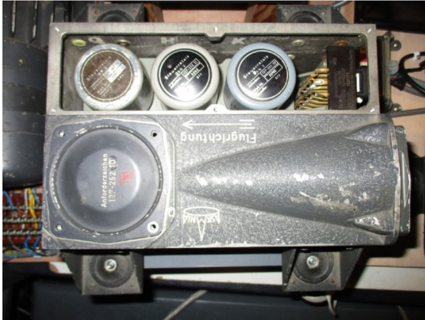
Fig. 7: Control unit. Visible: 3 Patin relays at the top and the roll damping gyro 127-262 10 at the bottom left.
