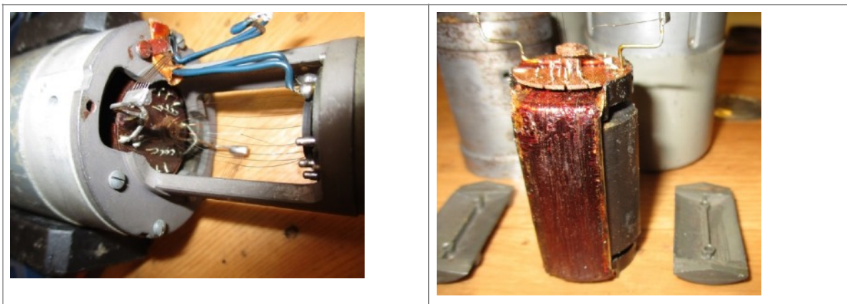
Fig. 10: A opened up Patin relay with burnt-out connecting wire (left) showing the four integrated galvanometer windings (right)
