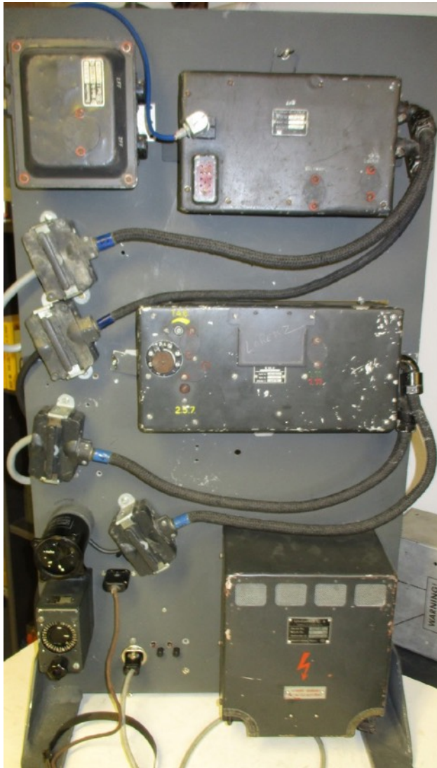
Fig. 24: Test board for the blind landing system with BI2, BI3f, converters and auxiliary equipment
