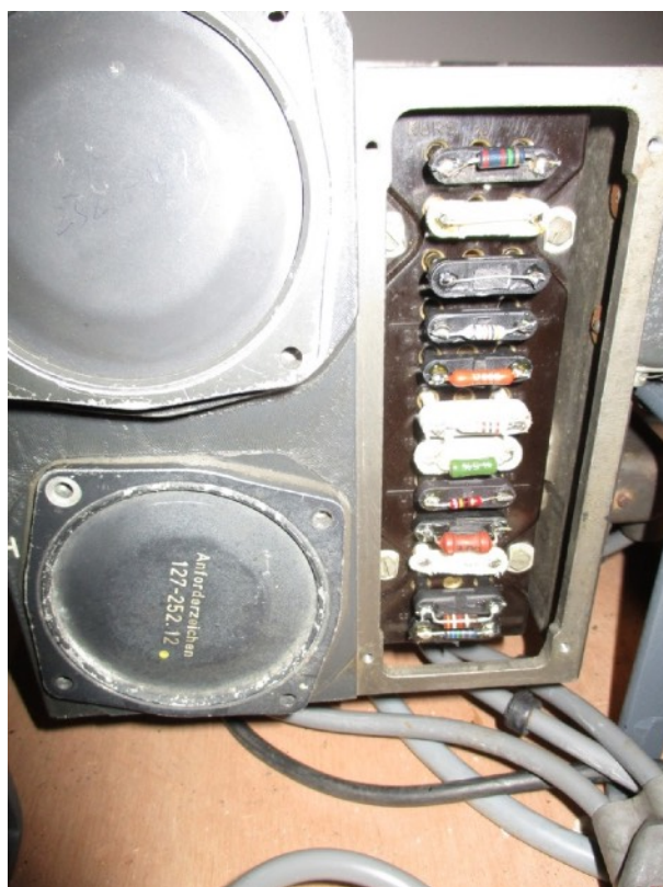
Fig. 9: Left the yaw and pitch damping gyros and on the right the control resistors to take into account the influence of the specific flight characteristics of an aircraft.
