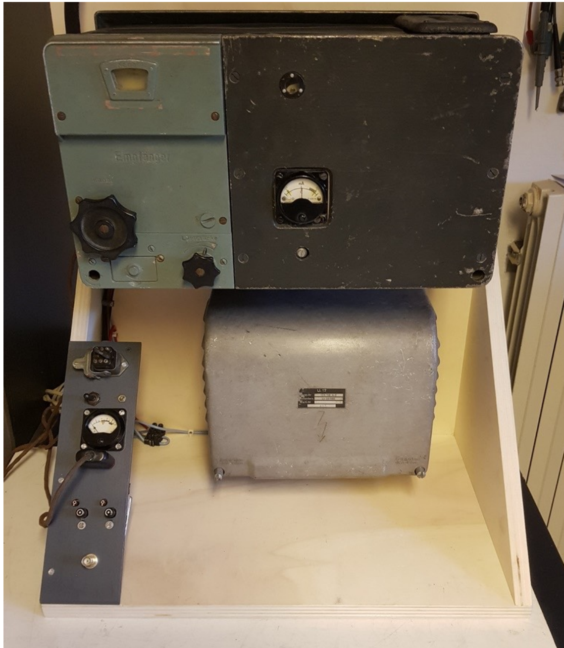
Fig. 15: Test board for FuG 28. The original receiver 17E is replaced by the equivalent receiver of the naval equipment Lo 10 UK 39 (painted in green)
