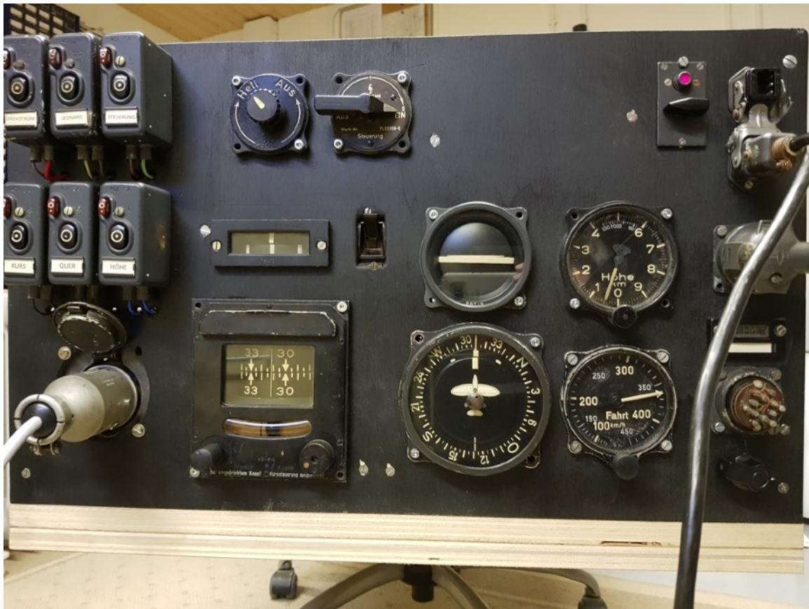
Fig. 1: Front panel of the "aircraft" in operating condition: altitude 500 m, speed 360 km/h, course 31.2° aircraft in horizontal position slightly rising. The red light, top right indicates that the remote control is on.
