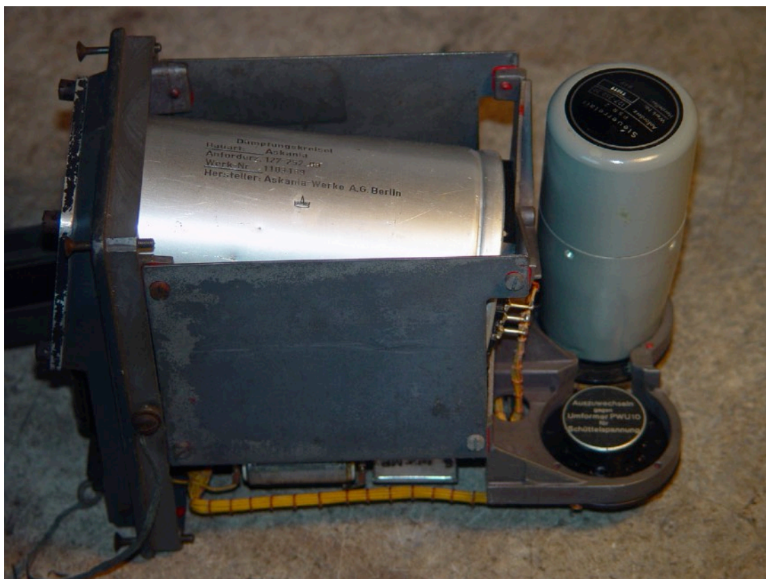
Figure 16: The interior of the SK 11 "Steuerkasten" with the "Deampfungskreisel" and "Steuerrelais" in place. Note the blind plug in socket where the PWU 10 "Schüttelumformer" could be plugged in.
