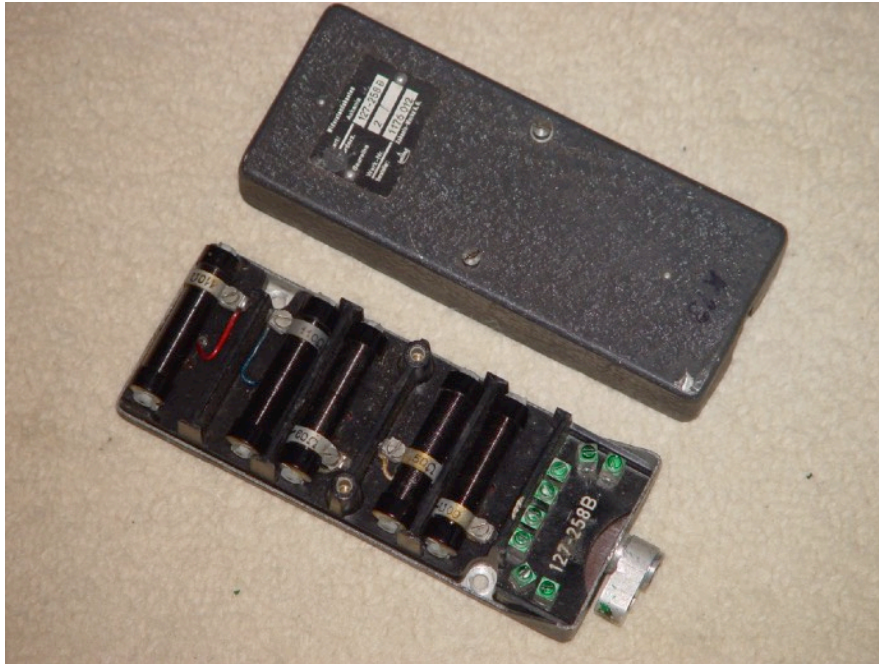
Figure 10: Early type "Widerstandskasten" made by Askania, opened up to show the resistors inside. Note the "K13" equipment code painted on the lid.
