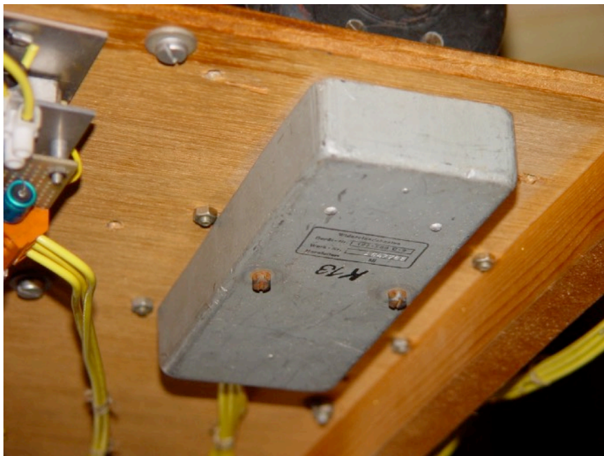
Figure 11: Later type "Widerstandskasten" made by Patin. Note the "K13" equipment code painted on the box
