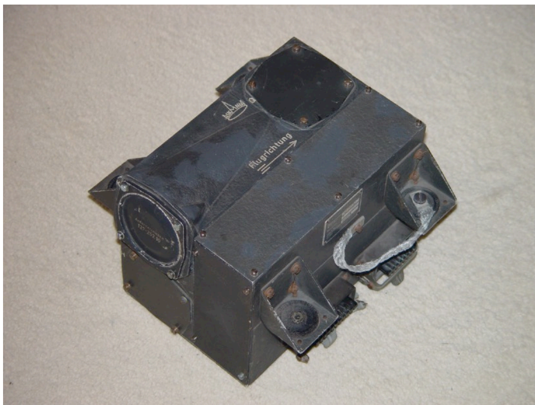
Figure 13: Early type Askania built "Steuerkasten" originally for the PDS system. Note the blanking plates where normally the damping gyroscopes for roll and pitch control would be inserted.
