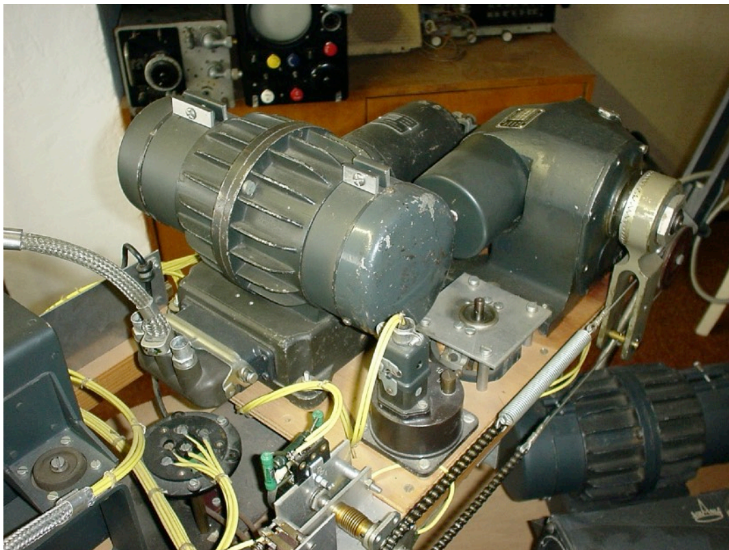
Figure 23: The "Leonard Umformer", "Rudergetriebe", "Drehstrom Umformer" and "Deampfungsregler" on the rear part of the turntable.
