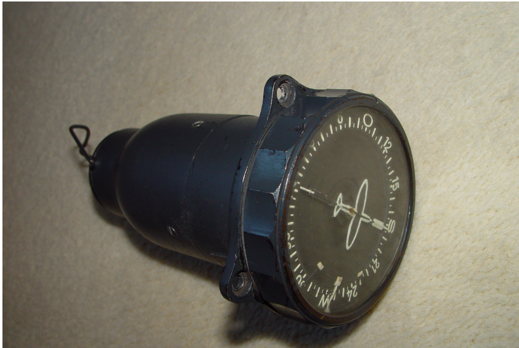
Figure 8: PFK/f2 repeater compass is a small diameter version of the f1. Note the knurled bevel for manually adjusting the set-point and the late-war "open" aircraft symbol of the indicator
