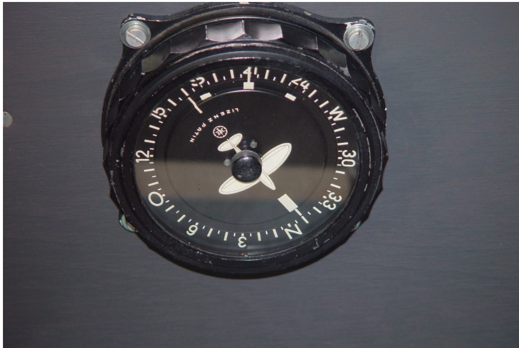
Figure 7: PFK/f1 repeater compass. The instrument has a knurled bezel that can be rotated to change the set point manually. Alternatively it can be connect to a course motor.
