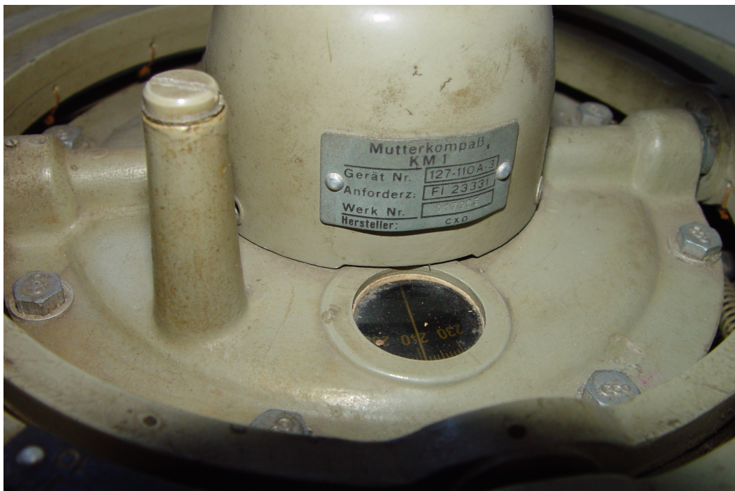
Figure 5: PMK-m date plate, note that it is alternatively denoted "KM-1" (Kompass Mutter 1)
