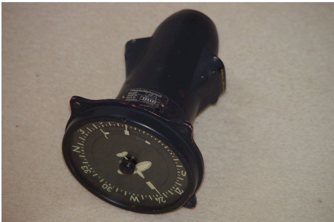
Figure 9: PFK-34 compass repeater. There is no knurled bezel for manual adjustment. The instrument has two connector sockets on the side of the housing.
