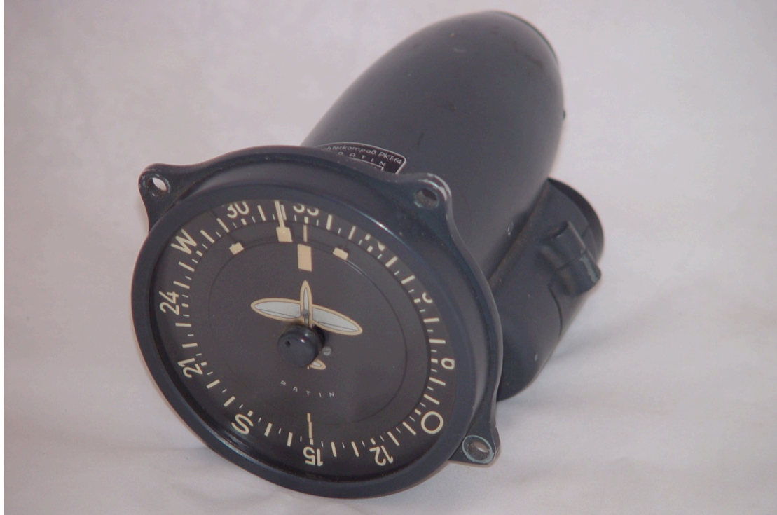
Figure 10: PFK-f4 compass repeater. Note the electric motor mounted under the instrument housing
