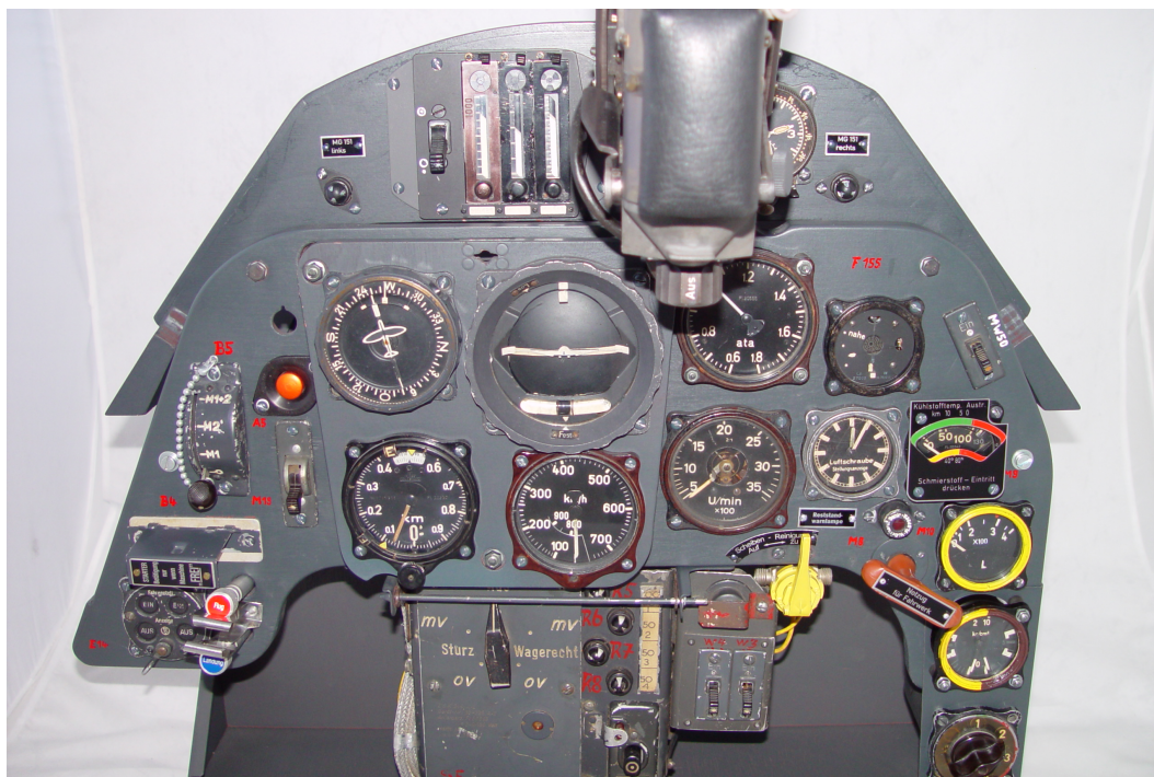
Figure 1: A Patin PFK/f2 compass repeater fitted to a Messerschmitt Bf109 G-6 panel
