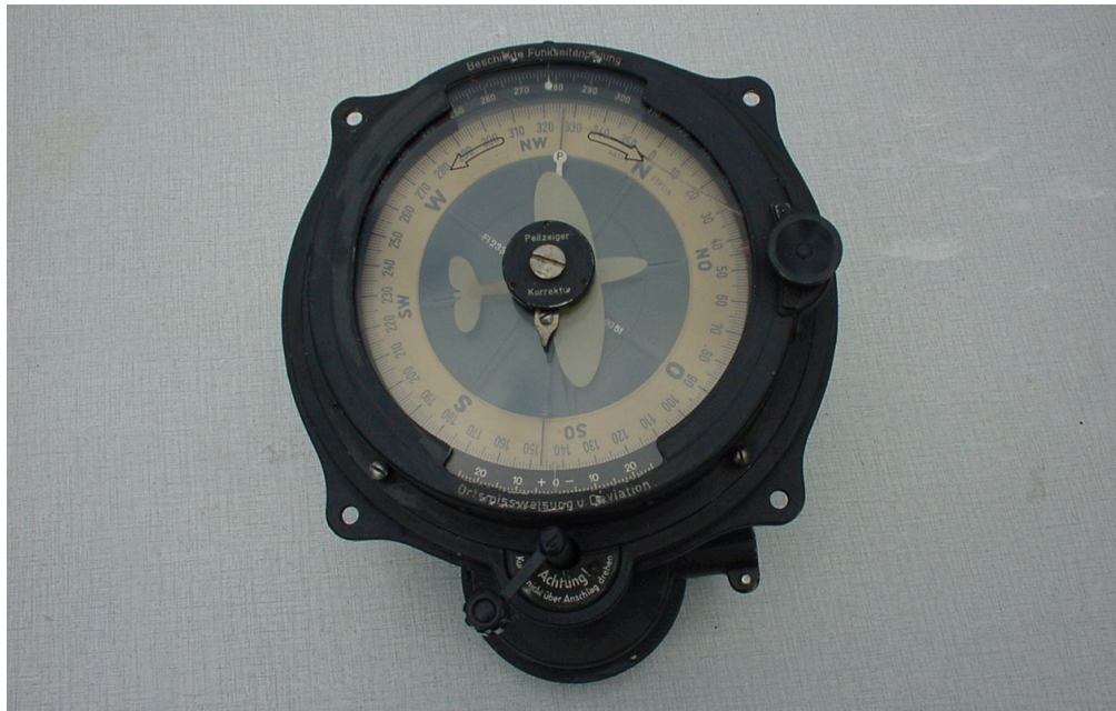
Figure 11: A complete PFA/R radio compass indicator. The central instrument is the PFK/p repeater compass.
