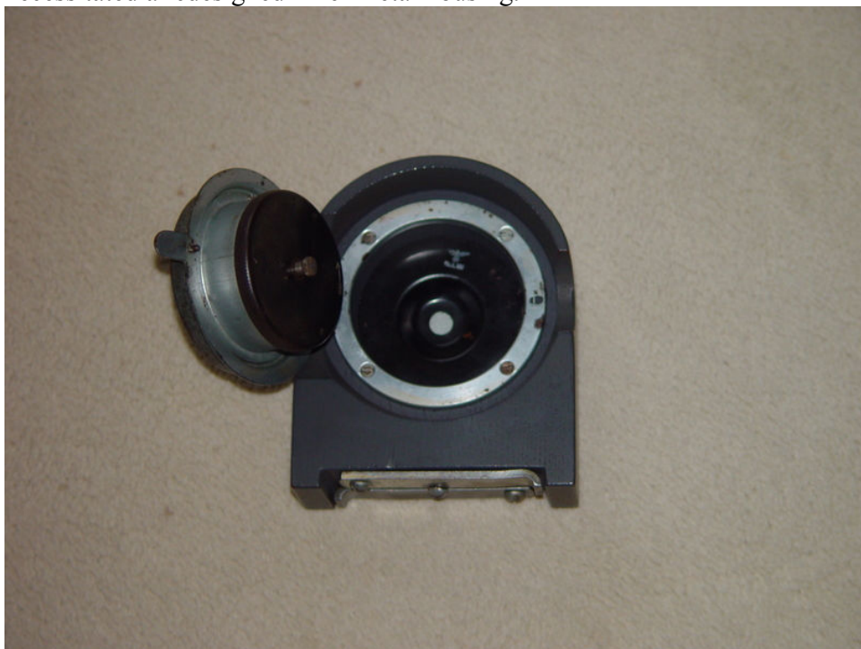
Figure 86: Opened clock revealing the metal ring containing serial number, year and army property statement. A Waffenamt stamp can be seen on the inner housing
