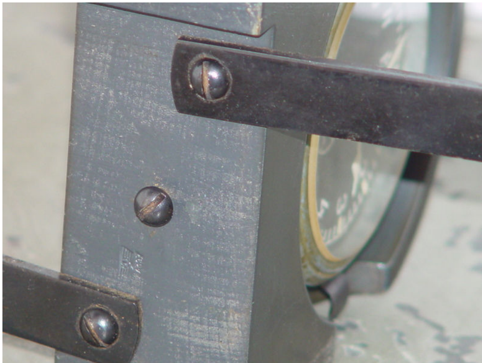
Figure 67: The two metal feet that could be extended to add stability
