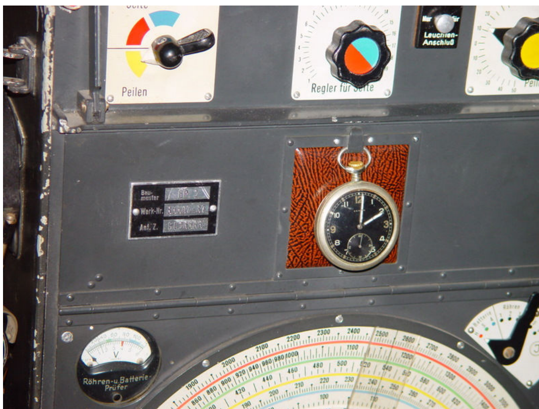
Figure 91: EP2 radio direction finder with hook and cushion for an Army "Dienstuhr"
