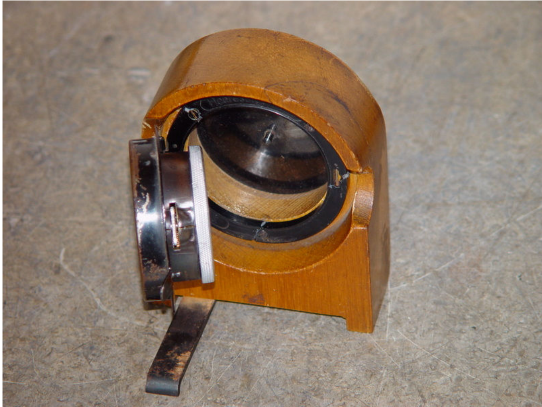
Figure 84: Opened clock revealing the bakelite ring containing serial number and army property statement. Note the time adjusting wheel on the side of the clock facing the viewer.
