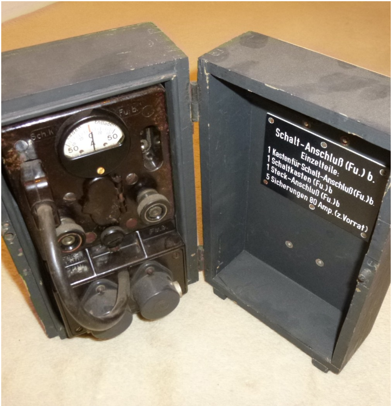
Schaltanschluß(Fu.)b which could be used to power the lights outside a vehicle, note the two Bosch sockets at the bottom
