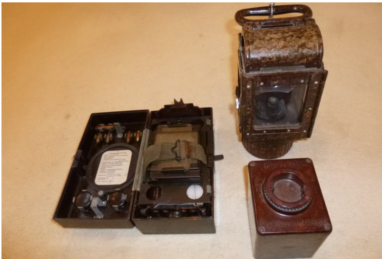
The "Laterne" set carried in the Fu71 consisted of a lantern, a carbide container and a spares box
