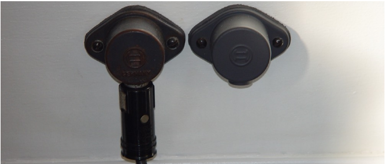
Bosch sockets and plug as fitted in vehicles
