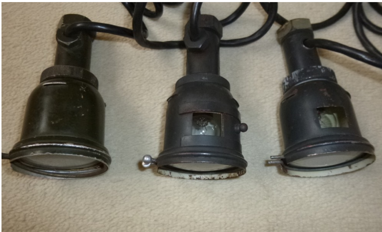
Three different shade types: (l) early type without "window", (m) type with sliding "window" and (r) type with open "window"
