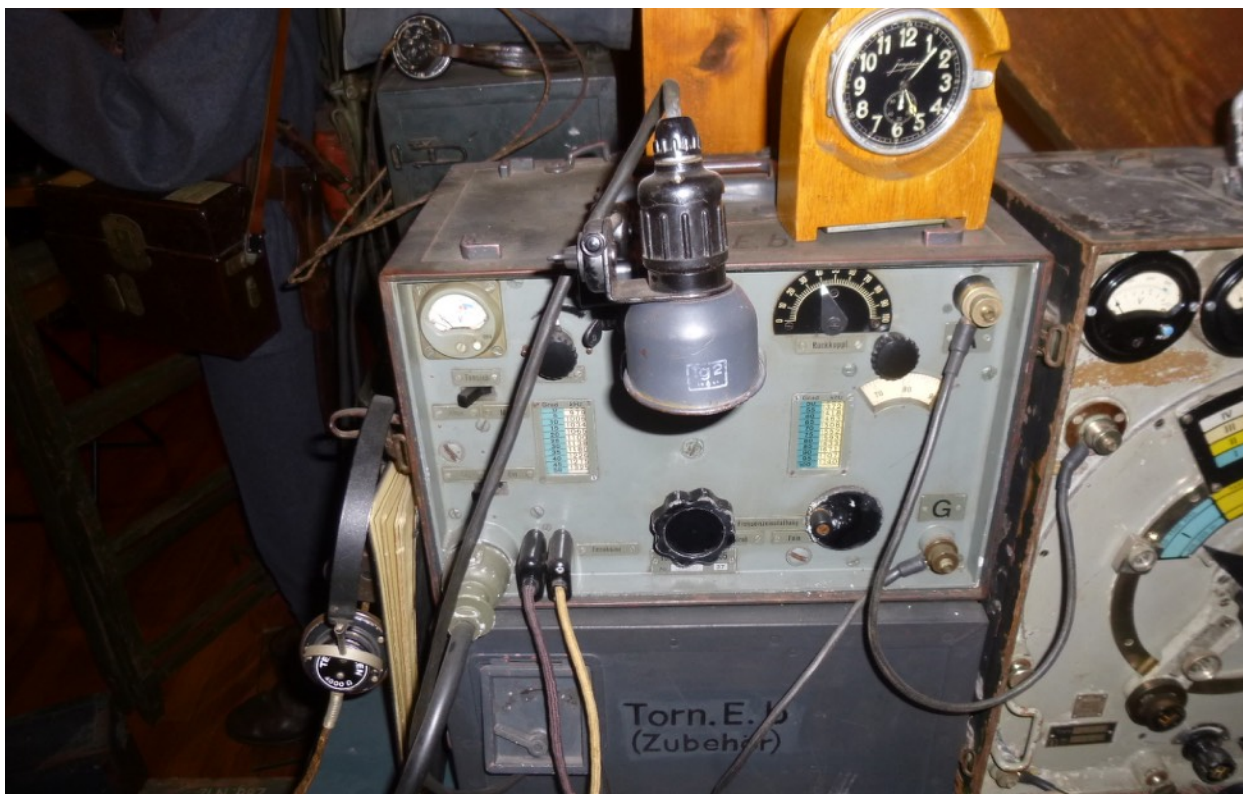
The Tg2 fitted to a Torn.E.b receiver. The cable is just the right length to reach the 2B38 battery in the "Zubehör" box
