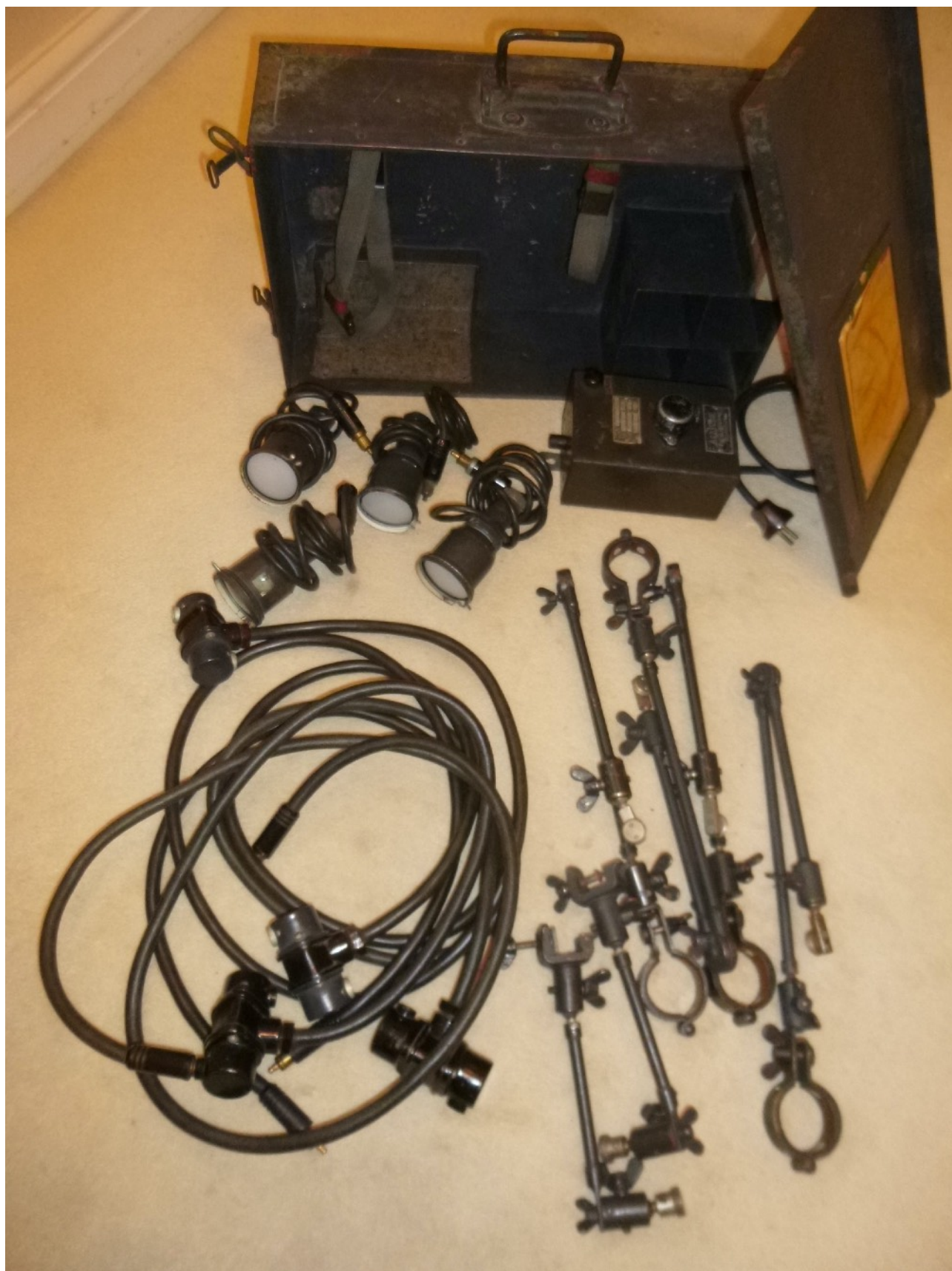
Contents of the FU82 "Zeltbeleuchtungs" set, showing lamps, transformer, extension cables, lamp brackets and swing arms
