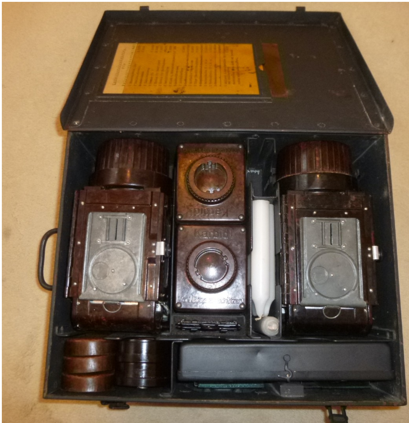
Fu51 box with two “Einheitslaternen”, carbide containers, candles and bunker lights and spare parts box
