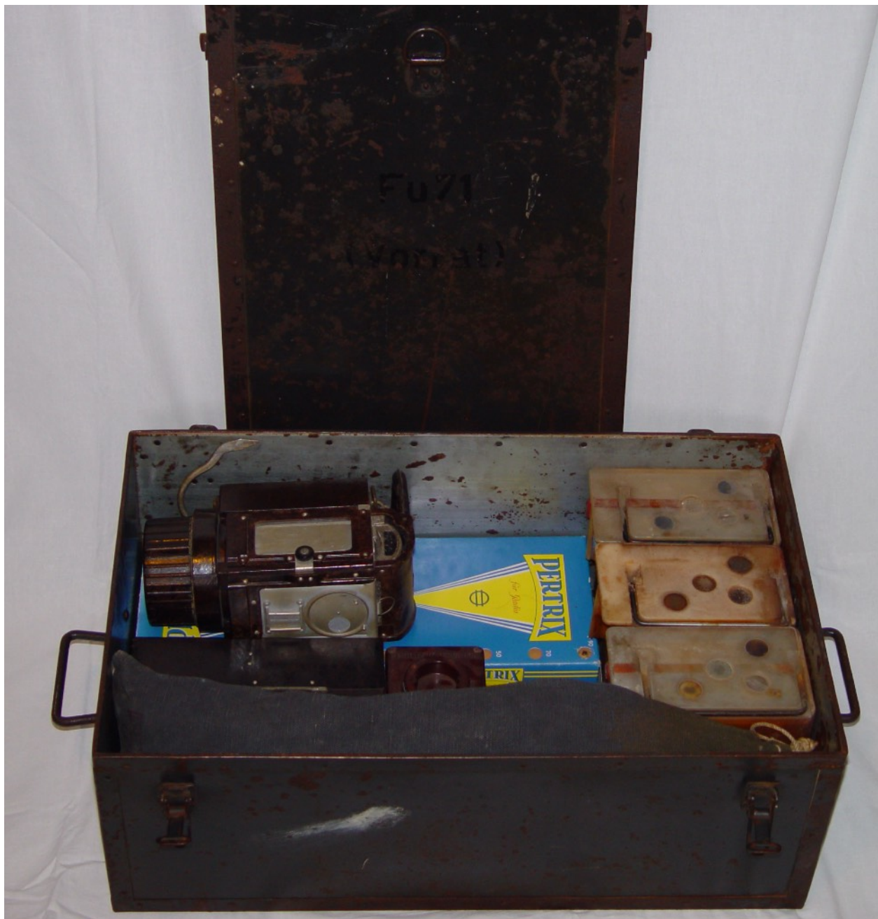
The FU71 case contained spares for the Torn.Fu.d2 radio equipment as well as a "Einheitslaternen" set
