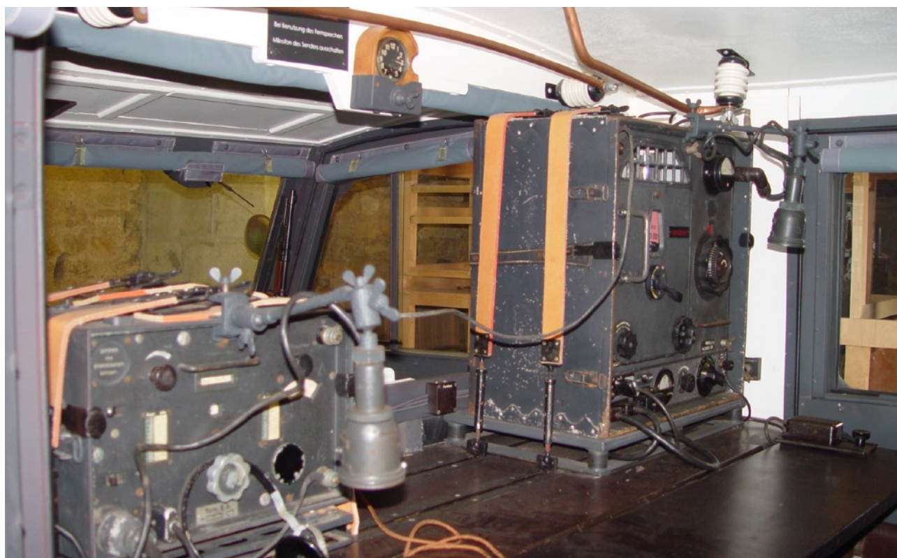
The Zbg.N12 lights used in a Kfz.17 radio car. The lamps mainly illuminate the table top in front of the radios to assist the reading and writing of messages forms etc.
