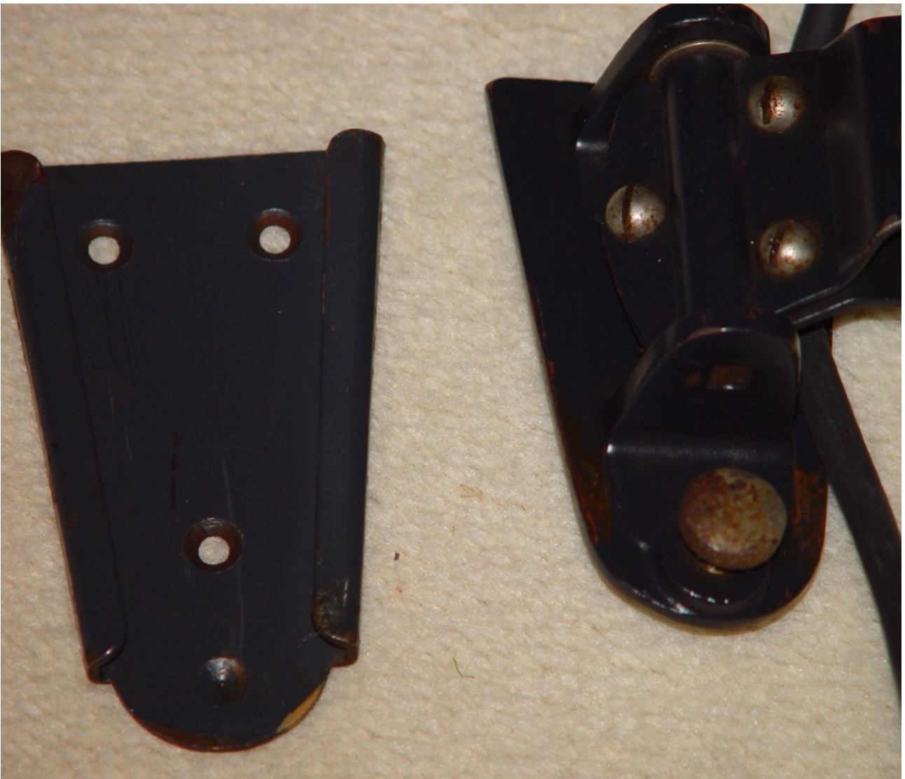
The “triangular” mounting plate and socket. The mounting plate slides into the socket and is secured with the crew knob.
