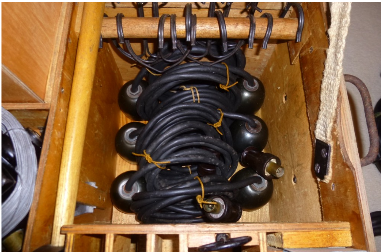
The six lamp sockets are stored in the bottom of the box
