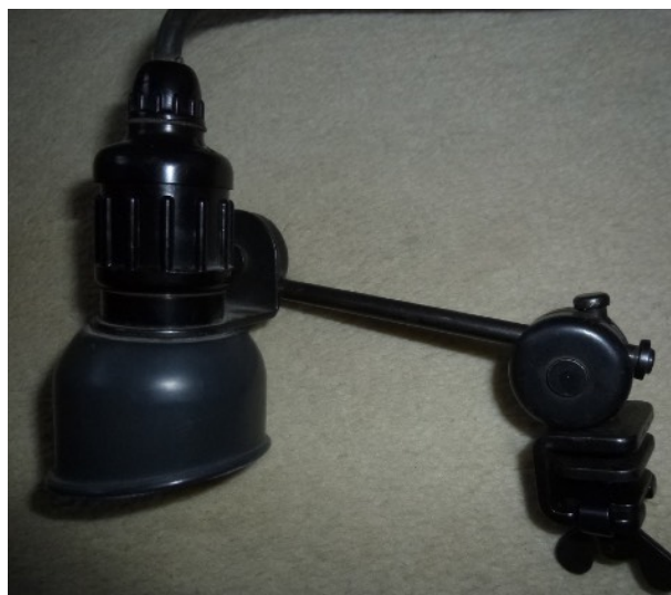
Two articulated joints and a clamp allow the lamp to be positioned in front of the receiver
