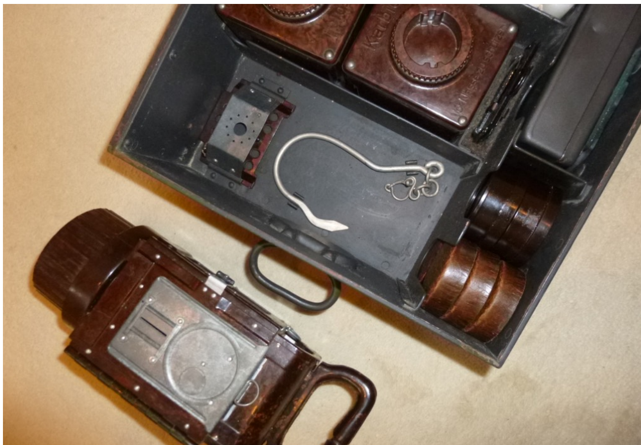
Fu51 with lantern removed showing the stowage of the hook and candle burner
