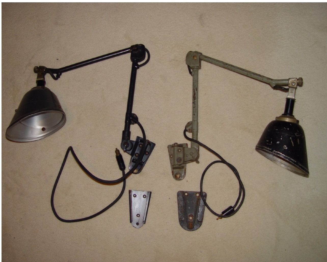
Midgard 12V radio vehicle lamps with mounting brackets. Pre-war manufacture (right) and wartime manufacture (left)
