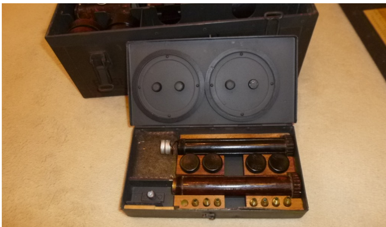
Spares box in the Fu51 with candle tubes, spare burners, gaskets and grease containers. In the Fu51 held an electric torch, a spare 4.5 V flashlight battery and bulb
