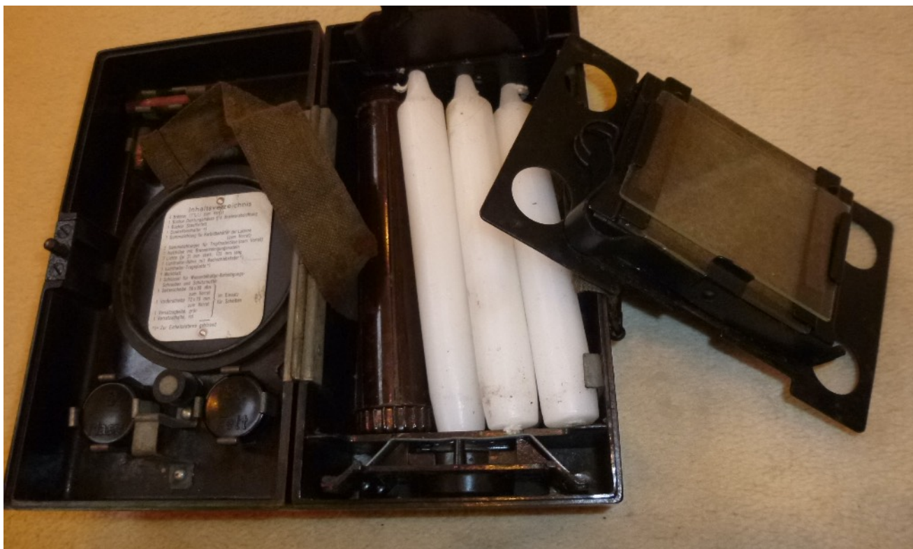
The spares box contains candle conversion with candles, spare glasses, blinds and filters and spare carbide burners and gaskets
