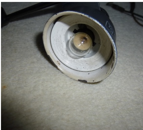
The white painted interior reflects the light of the 2V bulb
